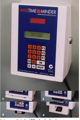
AMS Time-Minder's flagship clock, the TM06K, offers all the data-safe and error-free advantages of our previous model in a new compact modular casing. This clock connects directly to your network, can collect employee and job data via various inputs, has a built in bell timer, and your data is protected by powerful double back-up batteries.
